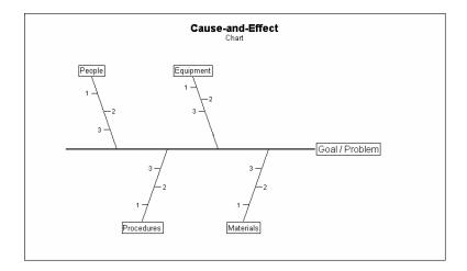
The fishbone chart organizes and displays the relationships between different causes for the effect that is being examined. This chart helps organize the brainstorming process. The major categories of causes are put on major branches connecting to the backbone, and various sub-causes are attached to the branches. A tree-like structure results, showing the many facets of the problem.
