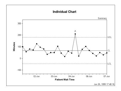
Individual charts plot the process results varying over time. Individual observations are plotted on the I chart, averages are not plotted on this type of chart. Individual charts are used to plot variable data collected chronologically from a process, such as a part's measurement over time.
