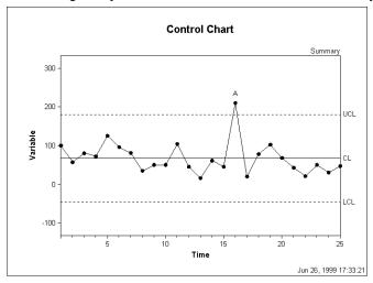
Control limits define the zone where the observed data for a stable and consistent process occurs virtually all of the time (99.7%). Any fluctuations within these limits come from common causes inherent to the system, such as choice of equipment, scheduled maintenance or the precision of the operation that results from the design. These normal fluctuations are attributed to statistical variability.
