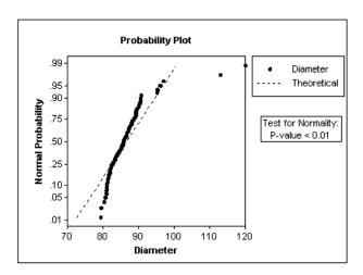
Although a probability plot is useful in analyzing data for normality, it is particularly useful for determining how capable a process is when the data is not normally distributed. That is, we are interested in finding the limits within which most of the data fall.
